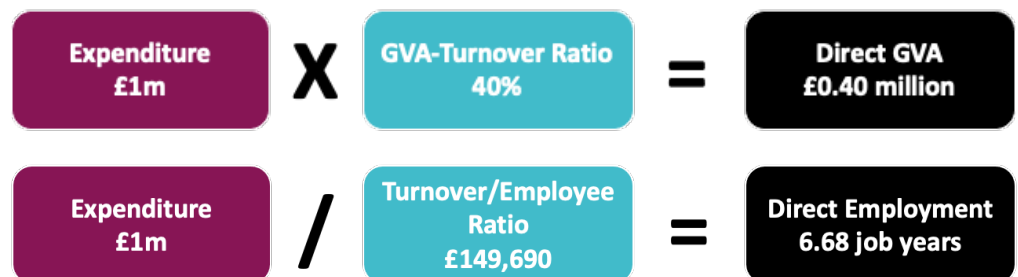
Figure 3.1 Direct Impact (Illustrative Worked Example)
